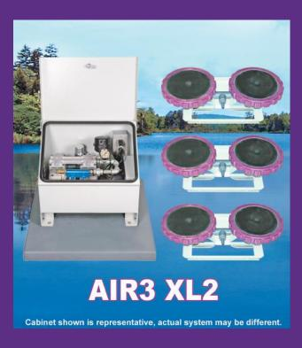
The Vertex Air3 XL2™ pond aerator is a super-efficient, affordable and safe system. In a typical pond, an Air3 XL2™ can aerate approximately 3-4 acres depending on shape, slope, oxygen demand and other factors. A 1/2hp (0.37kW) Brookwood™ SafeStart™ compressor, housed in our rustproof aluminum outdoor cabinet, feeds three bottom
