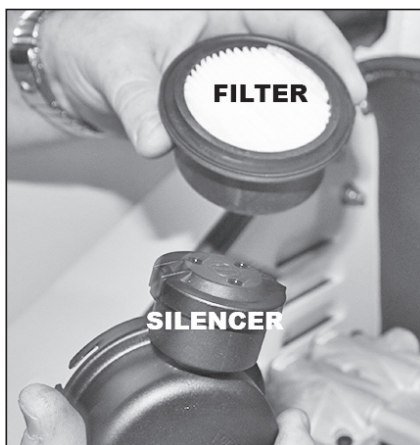
2 Remove old air filter Insert new air filter
