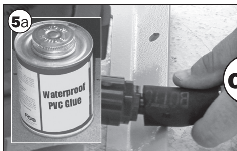
At the drop site, connect the tubing to the barbed fitting. Use PVC cement and let dry (recommended method), or...
