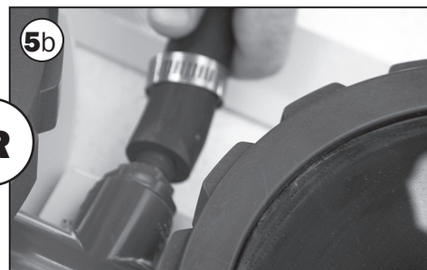
Connect the tubing to the barbed fitting with a stainless steel hose clamp.
