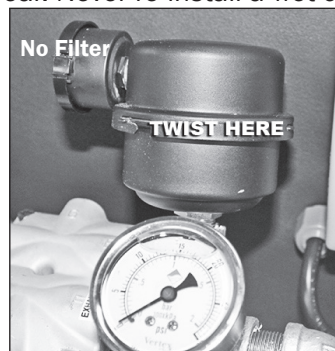
1 Twist to unlock air filter
