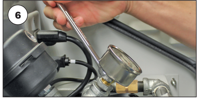
Remove the gauge using a 9/16" wrench
